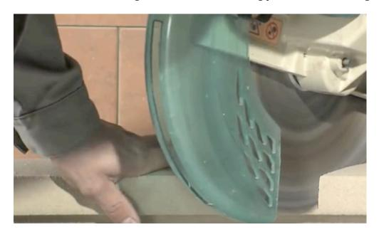
When cutting for corner finishes or for a window surrounds, cutting should be done at a 45-degree angle.
